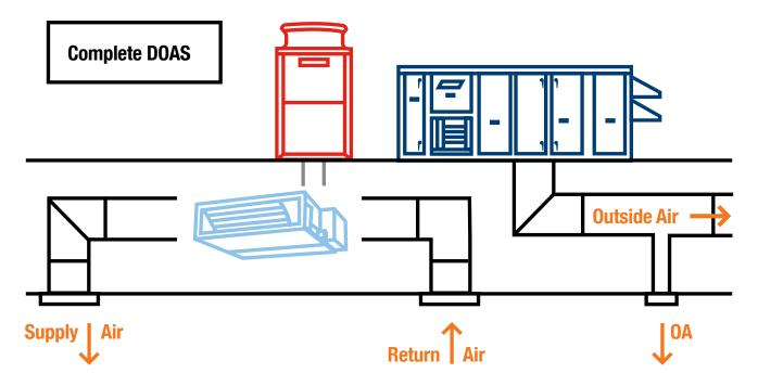
Decoupled designs that include a VRF system with an advanced refrigeration circuit can further increase efficiency as the DOAS conditions outside air to room neutral temperature.
