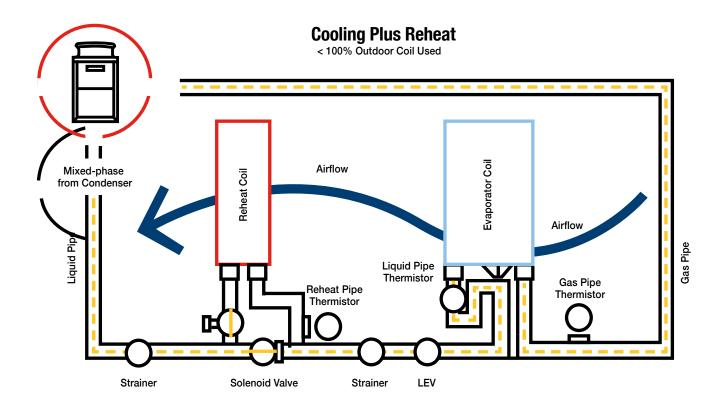
In the standard refrigeration circuit depicted above, a full-column of sub-cooled liquid refrigerant travels from the condenser to the evaporator coil while bypassing the reheat coil. Once the liquid reaches the evaporator coil, it is boiled into a low-pressure gas which then returns to the condensing unit.
